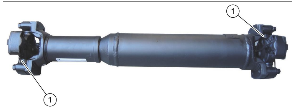
Fig. 26: Lubricating points of prop shaft
