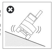
Level the ground in the machine's work area.
