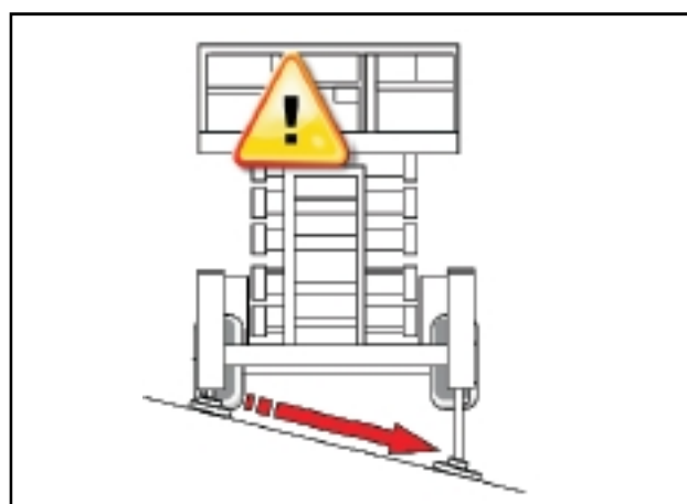
Figure 8.13 – Machine On Slope
