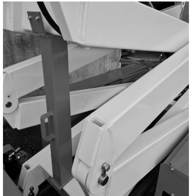
Figure 7.2 – Safety Prop in Support Position
