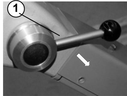
Control drive speed and direction of travel with the handle (1).
