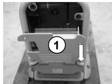
Open the screw cap (1) of the oil filler neck.
