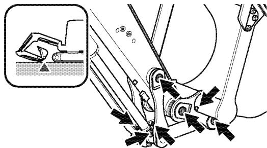
2. Clean the grease nipples indicated in the right figures and grease them using a grease gun.
