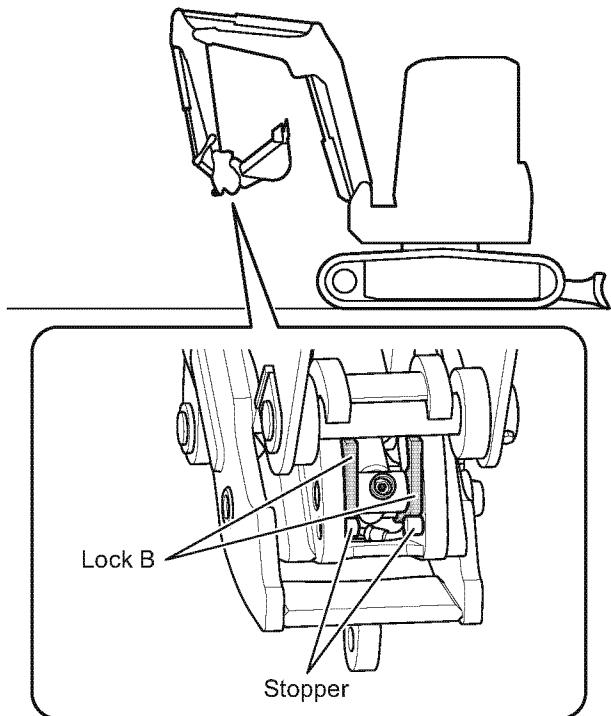
**8**. Make sure the attachment is securely mounted to the quick coupler and then press the power supply switch. The beeping sound will stop and the red lamp will go off.
