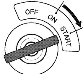
3. After the engine has started, release the starter switch key.
