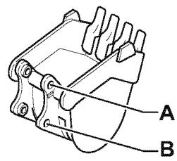
5. Clean the bucket boss section and install the O-ring.
