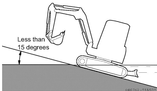
The limit of the water depth in which the machine can be used in is up to the center of the carrier roller.
