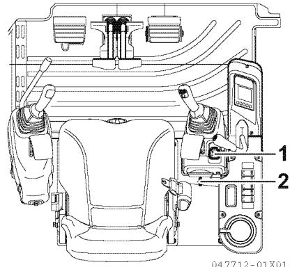
2. Turn the key in the starter switch **2** to the "ON" position and hold it in the position. An icon indicating that the engine glow plug is operating appears on the LCD monitor and disappears when the engine has been warmed up. Be sure to confirm that the icon has disappeared before starting the engine.
