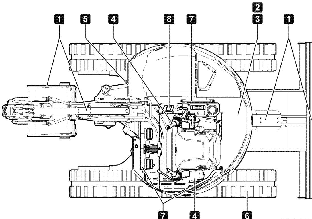
**1 Checking the implement, hydraulic cylinders, linkages, and hoses for damage, wear and loose connections**
