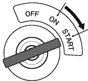
4. After the engine has started, release the starter switch key.
