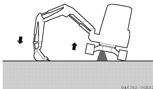
2. At a position that will be safe even if the machine should fall, measure the clearance between the bottom of the track frame and the upper surface of the shoe plate.
