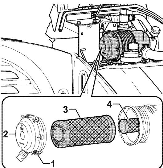
5. Blow dry compressed air [100 PSI (0.7 MPa) or less] from inside the element 3 along the pleats to initially remove the dirt. Then blow compressed air from outside the element 3 along the pleats to remove dirt. The blow compressed air again from inside the element 3.
