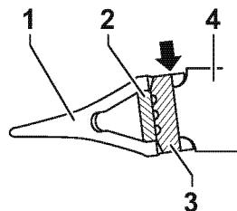
1. Strike out the locking pin 3, which connects the point type tooth 1 to the adapter 4, with a hammer and a tool applied to the pin for removal of it.
