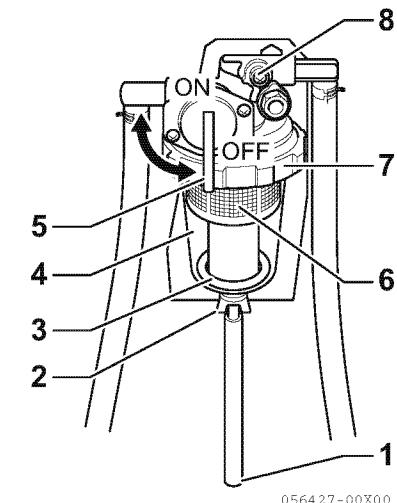
7. Check the O-ring and if it is damaged or deformed, replace it with a new one.
