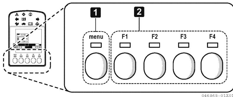
The function switches in the bottom part of the LCD monitor comprise 5 switches (a menu switch and F1 - F4 switches) and their functions change depending on the status of the machine or the screen currently displayed.
