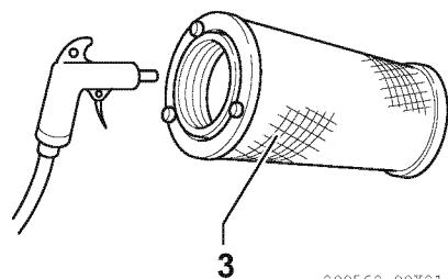
6. After cleaning, illuminate the element from inside with a light bulb to check it. If there are any small holes or thinner parts, replace the element with a new one.
