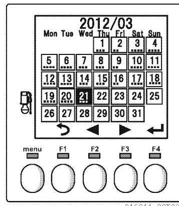
Operating hours are displayed with the corresponding numbers of dots.
