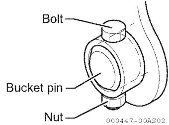
8. Install the bolt into the bucket pins **A** and **B**.
