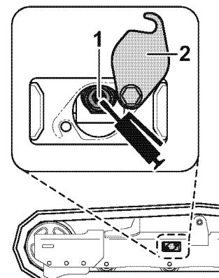
6. The tension can be adjusted until the clearance "a" is reduced to 0 in. (0 mm). If the tension is still loose after adjustment, the pin and the bush should be reversed or replaced because they are worn excessively. Ask your dealer to repair the track.
