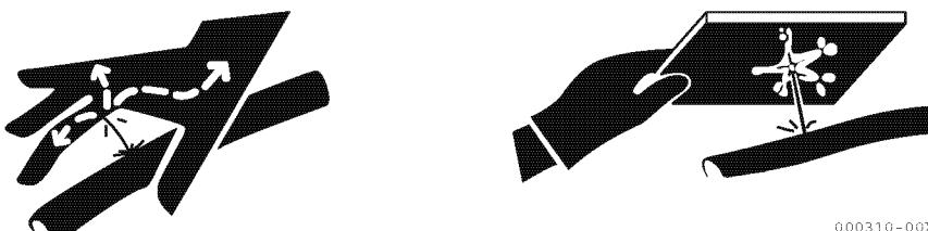
**Be careful when servicing systems under high temperature and high pressure**
