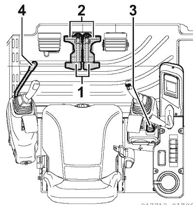
1. Set the left and right travel levers 1 or pedals 2 to the neutral position to stop the machine.
