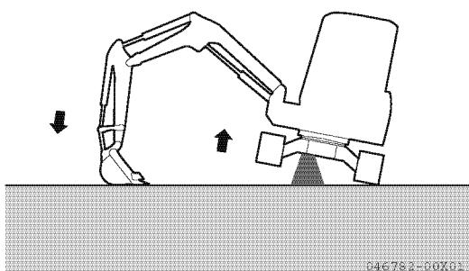
3. The tension is proper if the clearance (H in the right figure) between the outside rolling surface of the second track roller from the idler side and the inside surface of the rubber track is within the following range:
