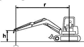
Note where application specifications conform to ISO standards. The weight of all lifting devices, including quick coupler, must be deducted from the value shown in the table to determine the net load that can be lifted.
