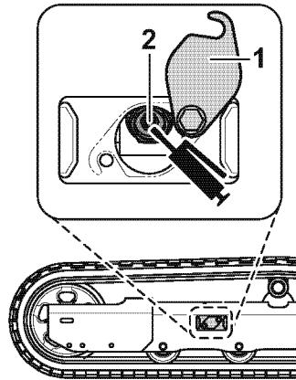
2. Raise the machine using the implement and inject grease through the greasing valve 2 using a grease gun until the rubber track tension is within the specified value of 0.3 to 0.5 in. (8 to 13 mm).
