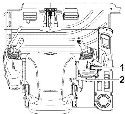
1. Turn the engine control dial **1** to the "RUN" direction.
