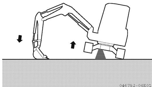
3. To check that the tension is proper, put down the machine and move the machine back and forth slightly.
