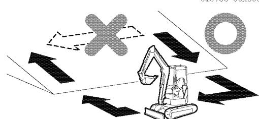
**Level the ground of the work site and the area within which the machine travels**
