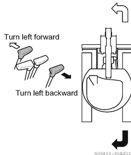
■ **Steering the machine while traveling
