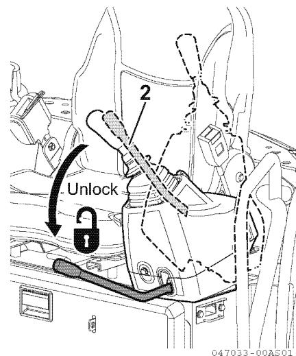
6. If the implement can go down on the ground with its self-weight, the accumulator is normal. If the implement cannot be lowered or stops along the way, the gas enclosed pressure of the accumulator for operation circuit could be reduced.
