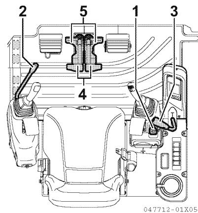
1. Turn the engine control dial **1** to the "RUN" position to increase the engine speed.
