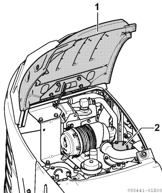
1. Open the bonnet B 1 and clean the area around the tank cover 2 on top of the hydraulic oil tank, using a cloth.
