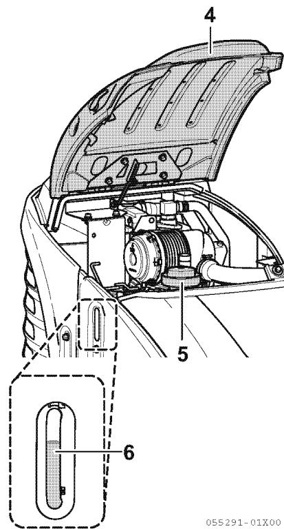
**2.** After refueling, securely retighten the fuel supply port cap, and close the engine hood B 4.
