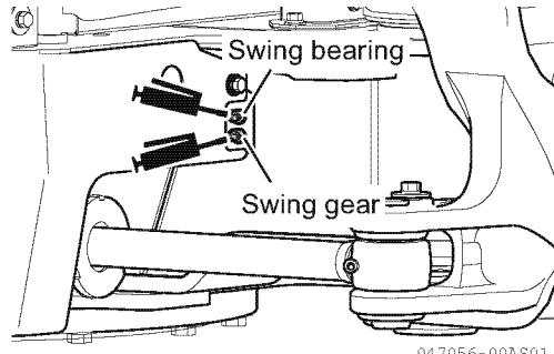
1. Grease the swing gear and bearing through the grease nipples indicated in the right figure, using a grease gun.
