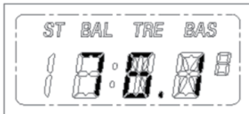
Frequency display (When stereo sound is not received, "ST" pict turns off)
